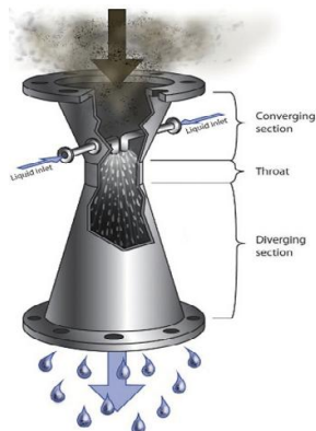
Capturing fine gases using venturi nozzles
