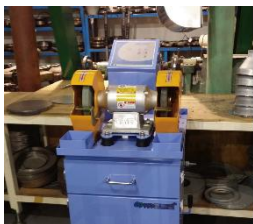
Dust collection during table grinder grinding
